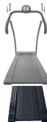
3. assemble the handrail: assemble the handrail into the frame, and fix it tightly by screw. (Note: Before set up the handrail, please screw the screws out of the frame. Then put away the handrail, screw the screws.)
