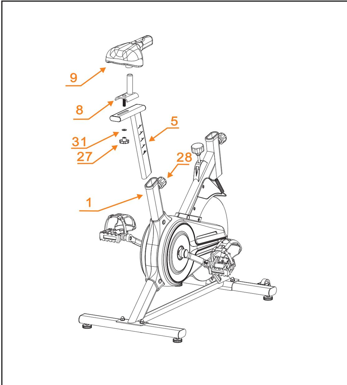
LOOSING LOCK KNOB (28) AND PULL OUT, INSERT THE SEAT POST (5) INTO THE MAIN FRAME (1).
