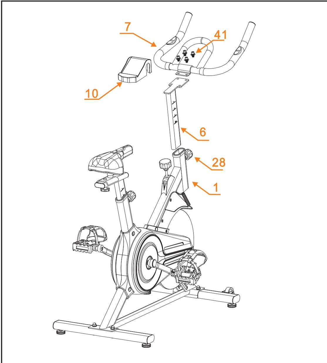
AS THE PICTURE SHOWS, FIX THE HANDLEBAR (7) WITH 2 SCREWS (4110) TO THE HANDLEBAR POST (6). THEN INSERT IT TO THE MAIN FRAME (1), USE THE PULL PIN KNOB (28) FIX TIGHTLY.PRESS IT DOWN TO THE HANDLEBAR.
