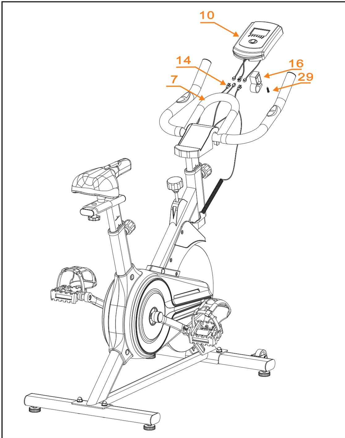
FIX THE PLASTIC MONITOR POST (16) TO THE HANDLEBAR (7) WITH SCREWS (29). PUT THE MONITOR (10) TO THE POST (16), THEN JOINT THE SENSOR WIRE (14). THE INTERFACES ARE MATCHING.
