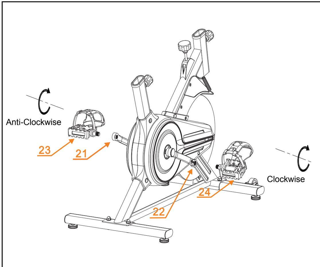
SCREW THE RIGHT AND LEFT PEDAL (23/24) TO THE LEFT AND RIGHT CRANK (21/22). SCREW 4-5 CIRCLES BY HAND, THEN FASTEN IT WITH THE WRENCH.
