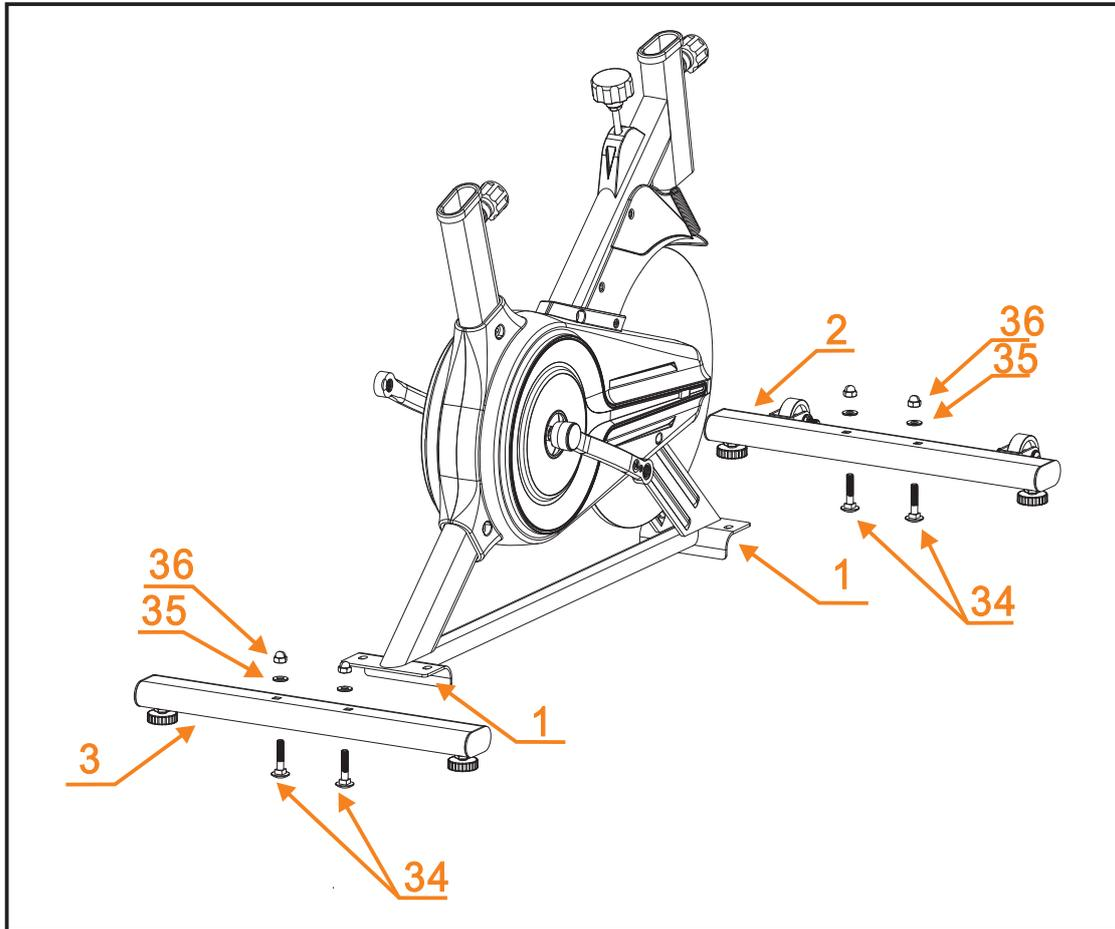
AS THE PICTURE SHOW, INSERT THE 4 CARRIGE SCREW (34) TO FRONT AND REAR STABILIZER, TOGETHER WITH THE FRAM (2/3). PUT THE GASKET IN IT (35), AND FIX IT WITH NUT BOLT (36).
