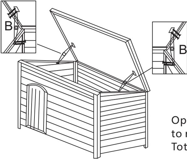
Open roof and fix 2x hinges. Secure one end of hinge to roof and the other end to the side panels as pictured. Total using 8x screw(B) in this step.
