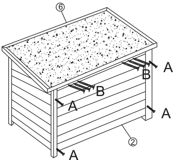
Secure back panel part② with 4x bolt&nut (A). Attach roof part⑥, secure by using 6x screw(B) at back.
