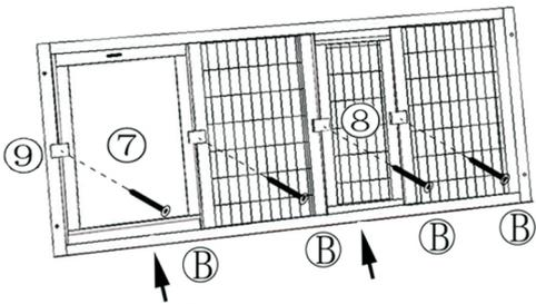
Attach part⑦ and part⑧ to part⑨, secure 4x part⑨ each with 1x screw(B) as pictured. Note: part⑦ and part⑧ are detachable entrance, not fixed.
