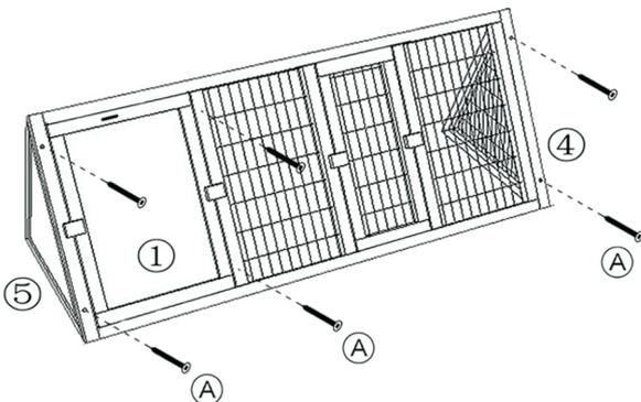
Secure left panel part⑤, middle panel part③ and right panel part④ by each using 2x screw(A), total 6x screw (A).
