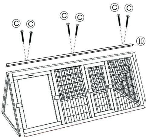
Attach part⑩ to the top, secure with 6x screw(C).
