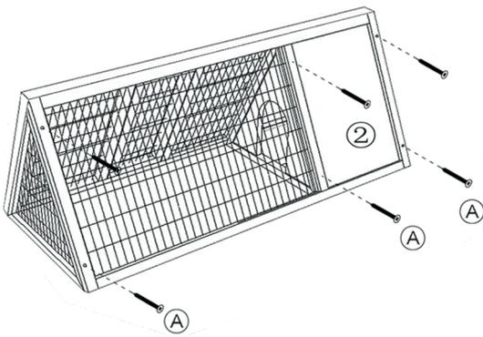
Secure back panel part② by using 6x screw (A).
