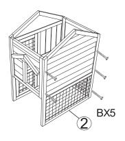
Secure back panel part② with 5x screw (B).
