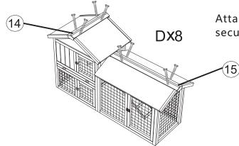
Attach part (4) and part (5) to roof respectively, each secured with 4x screw(D), total using 8x screw(D).
