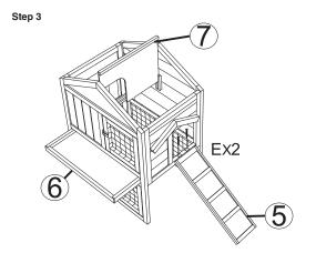
Put in metal tray part<sup>®</sup>, and insert part<sup>⑦</sup> from top as shown.
