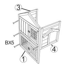
Attach side panel part ③ and middle panel part ④ to front panel part ①, secure with 5x screw (B).
