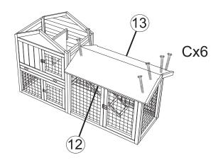
Attach roofs part 2 and part 3 , secure with 6x screw(C) as pictured.
