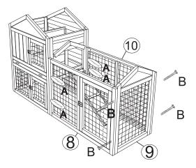
Attach part® and part⑩ to the main house finished in the above steps, each secured with 2x screw (A).
