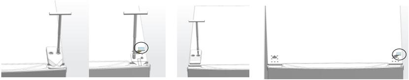
2. Remove and replace the pin on the other side of the upper hinge using a spanner.
