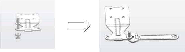
3. Remove and replace the axis sheath from right to left.
