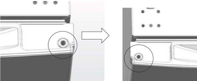
4. Remove the door and place it on a padded surface, and then remove and replace the limited block from right to the left using a screwdriver.
