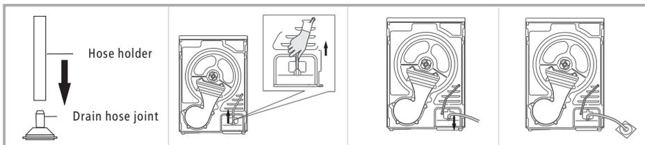
Pull up the drain hose joint
