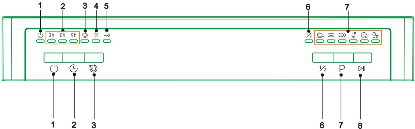
1. Power Button and Indicator: Switch On/Off the appliance, the indicator lights up when the power is on.
