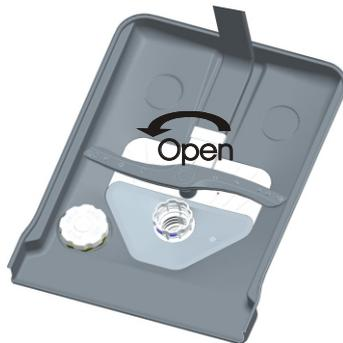
Step 1: Turn the filter in anti-clockwise direction,
