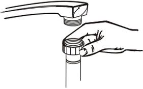
Connect the cold water supply hose to a threaded 3/4(inch) connector and make sure that it is fastened tightly in place.
