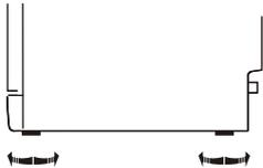
Once the appliance is positioned for levelling, the height of the dishwasher may be altered via adjustment of the screwing level of the feet. In any case, the appliance should not be inclined more than 2°.
