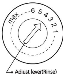
Turn the rinse aid indicator dial to a number between 1 and 6. The higher the number, the more rinse aid the dishwasher uses. If the dishes are not drying properly or are spotted, adjust the dial to the next higher number until your dishes are spot-free. Reduce it if there are sticky whitish stains on your dishes or a bluish film on glassware or knife blades.
