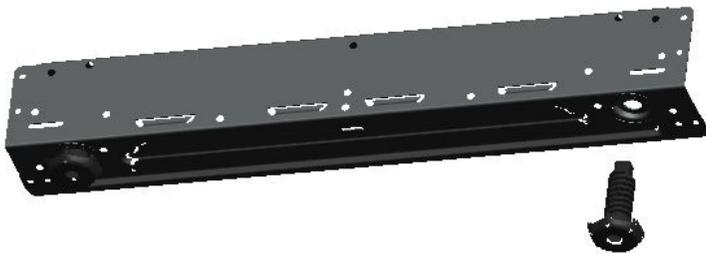
In order to prevent tipping of the appliance, this stabilizing means must be installed. Using ground screw 2 to mount the anti-title bracket 1 on the ground showed as the below picture .
