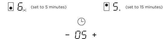
• Once the countdown timer expires, the corresponding zone will switch off. Then it will show the new min. timer and the dot of corresponding zone will flash.
