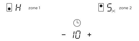
• When cooking timer expires, the corresponding cooking zone will be switch off automatically.
