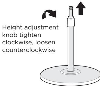
Height adjustment knob tighten clockwise, loosen counterclockwise
