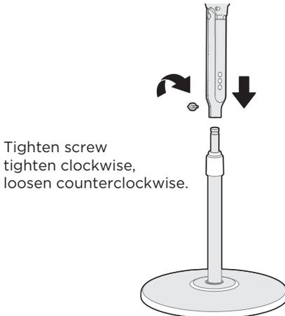
Tighten screw tighten clockwise, loosen counterclockwise.
