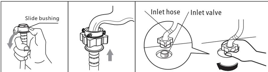
5. Press slide bushing, insert inlet hose into connecting base
