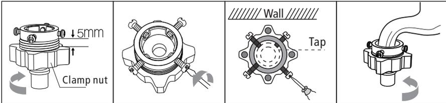
1. Loosen clamp nut to show 5mm thread
