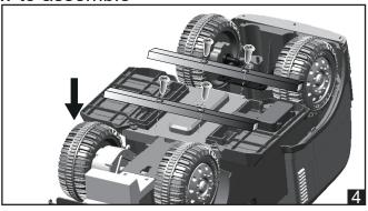
4. Assemble two square tubes to the car body according to the arrow, then use 4pcs M4\*12 screw to tighten.
