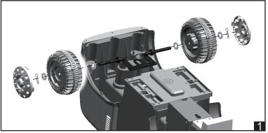
1. Add gasket, wheel, gasket, cotter and wheel cover to each side of steering wheel one by one. (P1)
