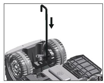
5. Insert the steering lever to the car body according to the arrow, then turn over body by holding up steering lever, in order to it falls.
