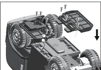
3. Connect two terminals of car body and foot rest, then assemble two foot rest according to the arrow and use 10pcs M4\*12 screw to tighten. (P3)
