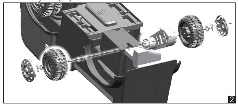
2. Add one gasket to rear axle from the right side, insert rear axle to car body. Add motor to the right side and add gasket to the left side. Then add wheel, gasket, cotter and wheel cover one by one. (P2)
