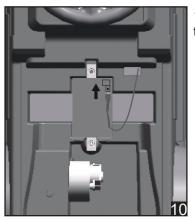
10. Connect the red line to the red terminal of battery. (P10)
