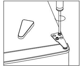
3. Remove the hole cover with a flat screw driver.
