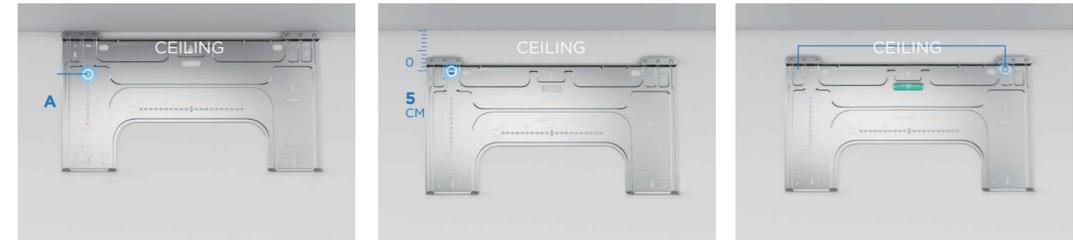
**STEP 1:** Mark the **SPOT A** according to the instruction of scale-on-plate
