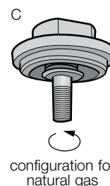
top hat nut assembly fully screwed down
