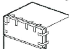
2) Dismantle top hinge cover, top hinge and hole cap of the other side.
