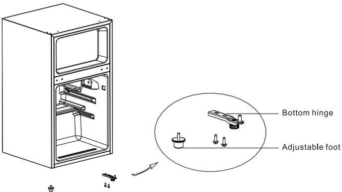
5) Exchange the installation position of bottom hinge and adjustable foot, then fix them respectively. Remove the hinge sleeve pipe of the refrigerating chamber door, and install it on the other side. Remove the hinge sleeve pipe of the freezing chamber door and install it on the other side.
