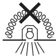
Luminaires not suitable for covering with thermally insulating or other material.
