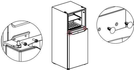
7) Take out the left upper hinge, left upper hinge cover, and right decorative cover from the accessory bag, install the freezer door on the middle hinge, and install the left upper hinge, left hinge cover and hole cap. Finally, install the right decorative cover on right side of end cap of freezer door..
