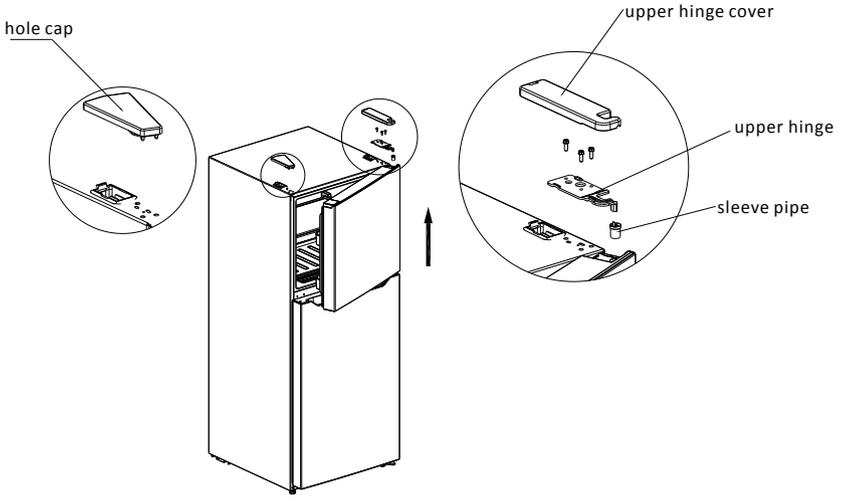
3) Remove the hole caps, fitting screws of middle hinge and middle hinge, then uplift the refrigerator door until it is separated from cabinet completely.
