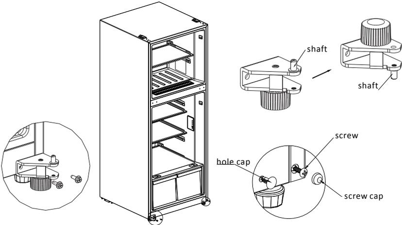
5) Dismantle the stoppers, sleeve pipes of both refrigerator door and freezer door, install them on the other side of both doors; exchange the installation position of sleeve pipe and hole cap on upper end of refrigerator door; remove the left decorative cover of freezer door, and move the sleeve pipe
