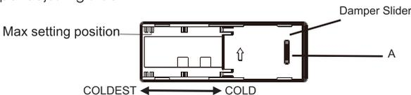
The temperature inside the freezer can be adjusted by changing the position of the damper slider. The initial position of the damper slider is at position A. If lower temperature inside the freezer is required, you can adjust the damper slider from the position A to left side.
