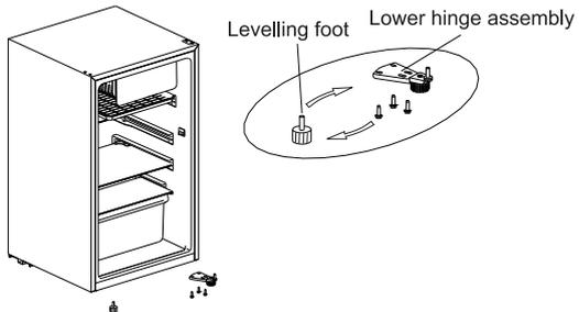
4) Install the door on the lower hinge assembly, and then install the upper hinge, hinge cover, shaft sleeve, pins and hole cap in sequence.
