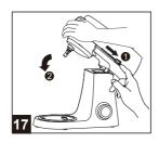
Release lock lever right, press down the head of the mixer.
