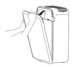
3 Take out the HEPA filter Hold both sides of the HEPA filter with both hands, and take it out
