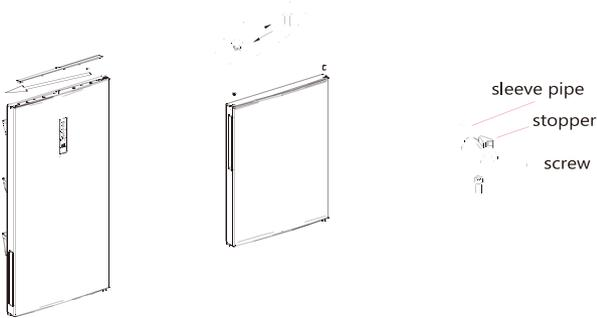
6. Put the freezer door on bottom hinge, install the middle hinge, the screws and the screw hole caps.
