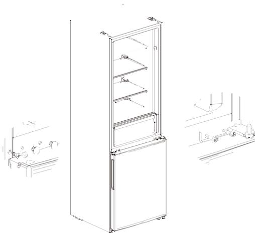
4. Dismantle the bottom hinge, hole caps and screws, Install the bottom hinge shaft on other side of the bottom hinge, then install the hinge on the other side.
