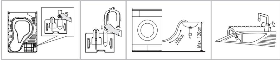
Use a pliers to remove the drain hose from the hose connector.
