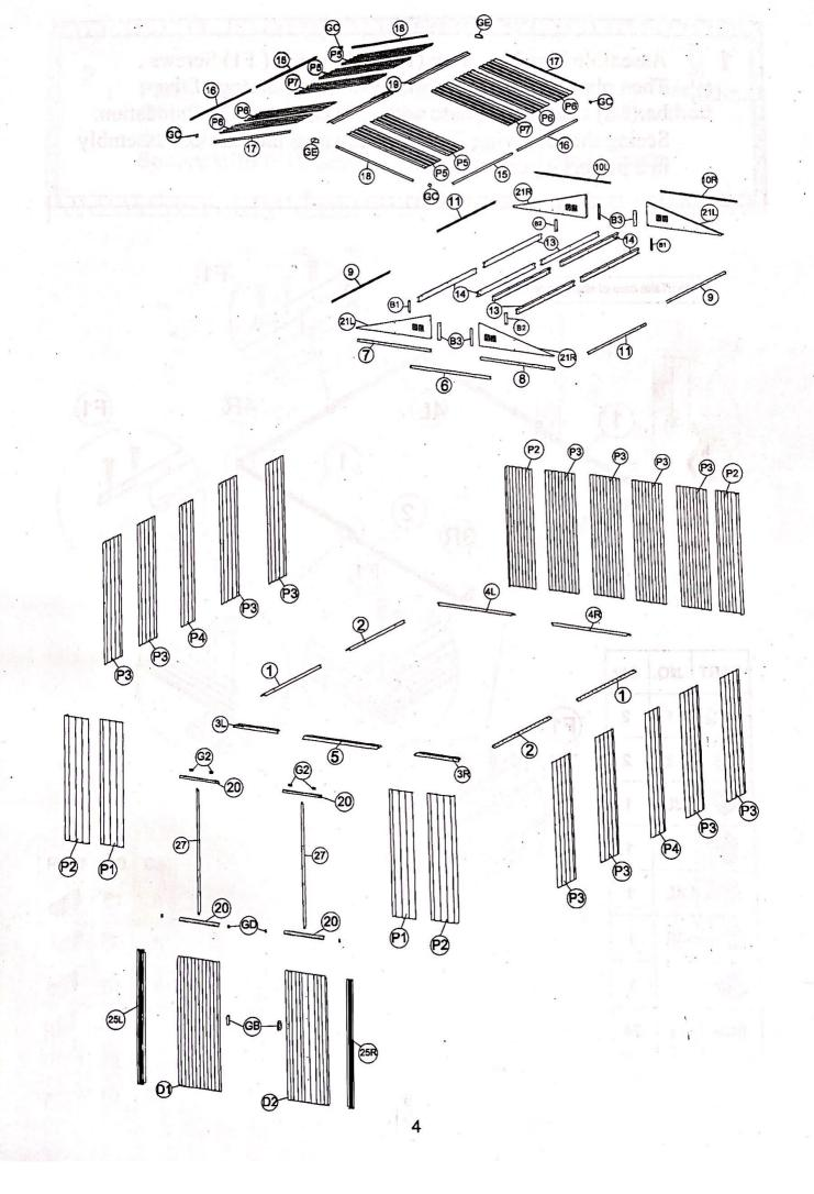
Assemble base bars from (1) to (4R) with (F1) Screws.
