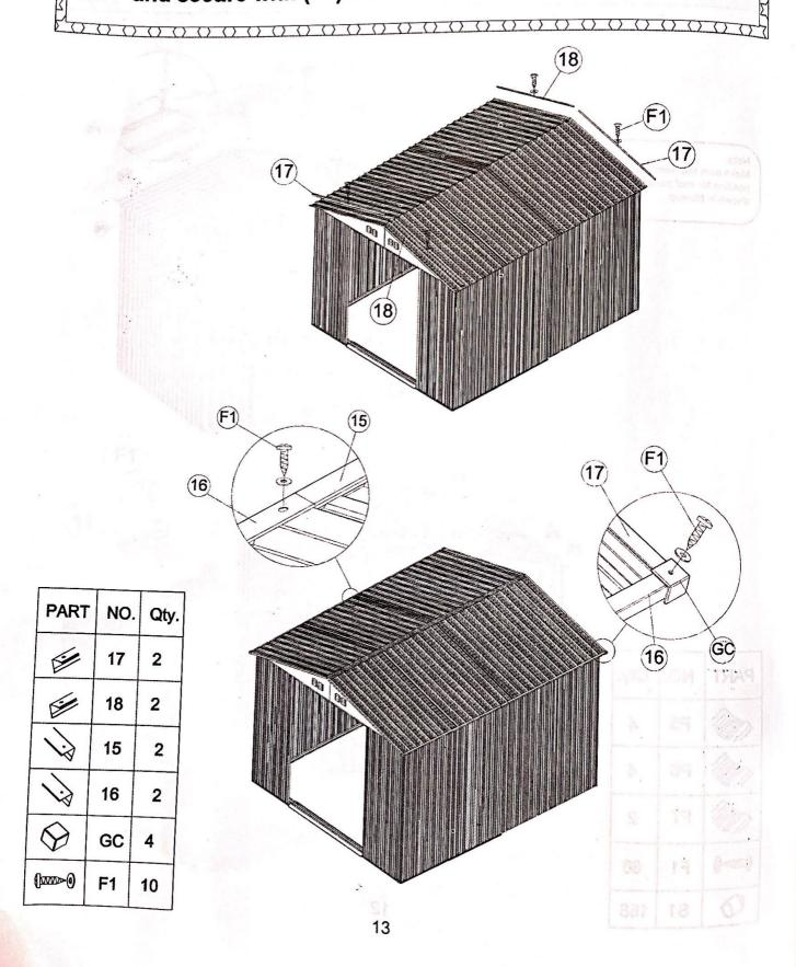
Place two pieces of the roof flashing center (19) on top of the roof panels, the flashing end cap (GE) to the front & back top of the roof and secure with (F1) screws with washers. See figures below.
