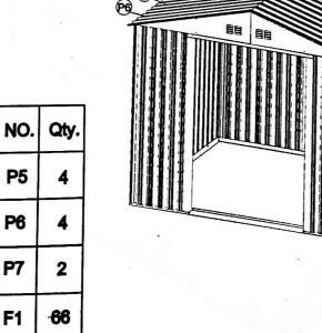
Assemble the roof flashing (15)(16), and (17),(18) with roof panels, secure with (F1) screws with washers. Then place 4 piece of top corner (GC) on the roof flashing joints. and secure with (F1) screws with washers.
