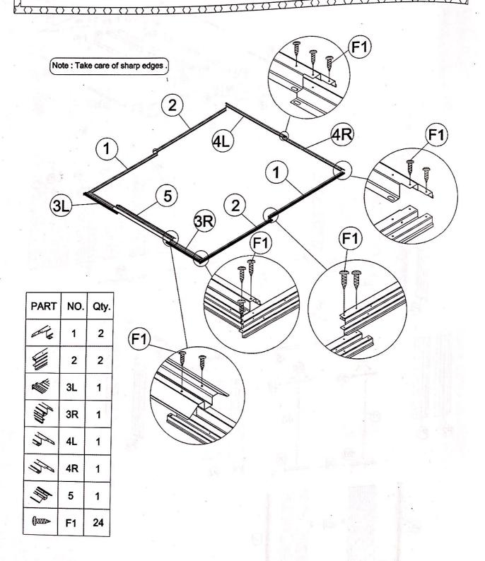
Place the wall panel (P1),(P2),(P3),(P4),on the base bar (1), (3L),(3R), (4L),and (4R) as showing .Side wall of the shed line up the Holes With base bar. Secure with (F1). Screws with washers from outside.
