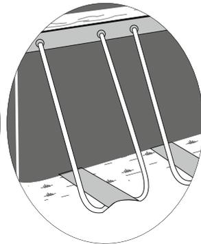
Do not assemble on soft lawn. If you must assemble the pool on a soft surface, timber boards must be placed under the feet of the vertical supports to spread the load.
